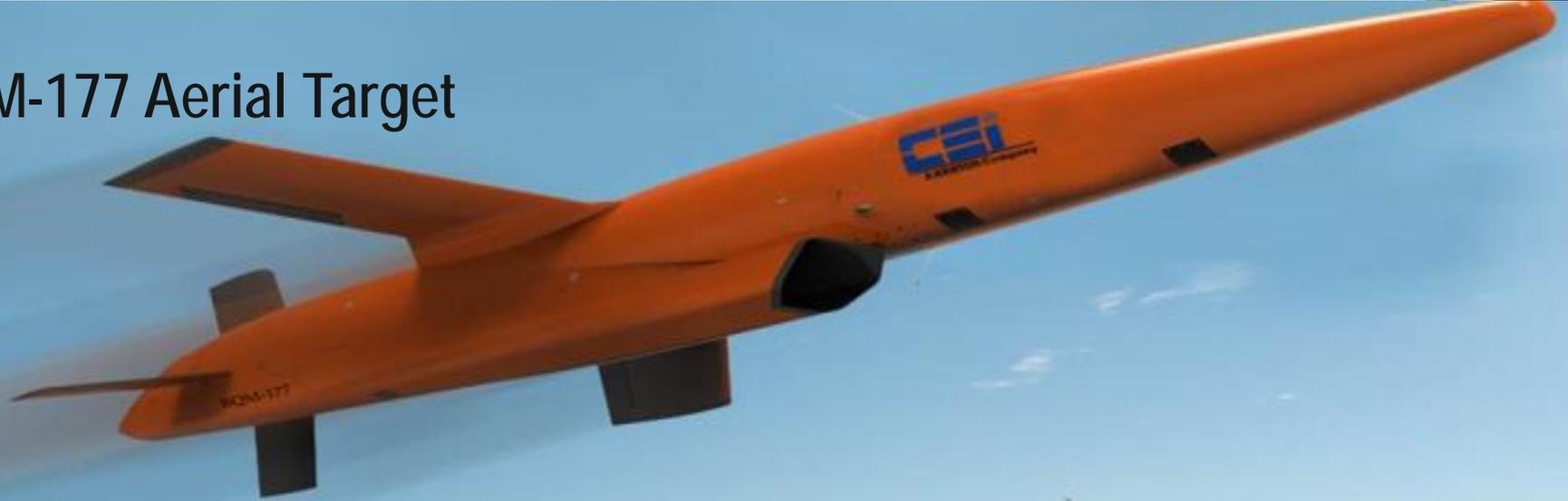
Kratos/CEI's BQM-177 provides the world's most advanced and realistic anti-ship cruise missile threat emulation with Low Altitude Cruise 10 feet above the water at .90 Mach.
