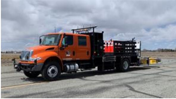
**Autonomous Truck-Mounted Attenuator now deployed in Southern Colorado paint striping operations**
