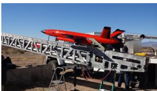
Kratos Firejet MQM-178 on its Pneumatic Launcher
