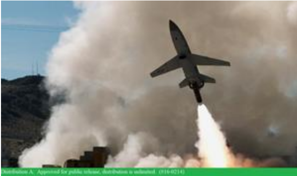
Kratos Mako Tactical UAS during Rocket Assist Take-Off (RATO) Launch
