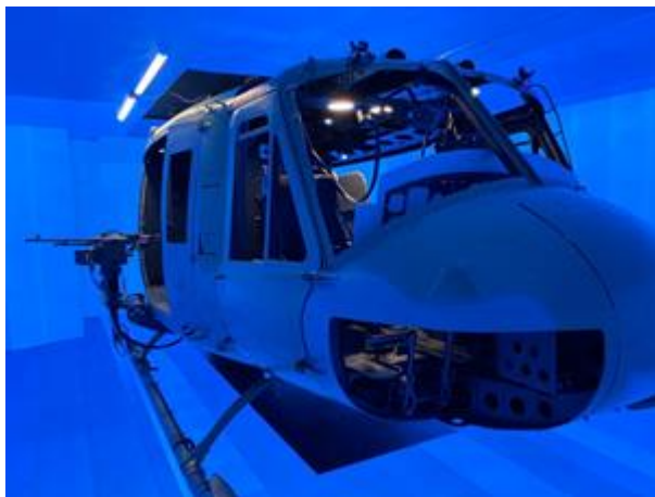
An actual UH-1 helicopter inside the blue electroluminescent interior of the Kratos immersive environment.
