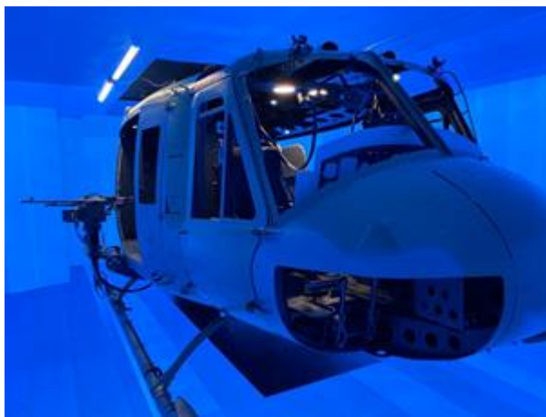
An actual UH-1 helicopter inside the blue electroluminescent interior of the Kratos immersive environment.
