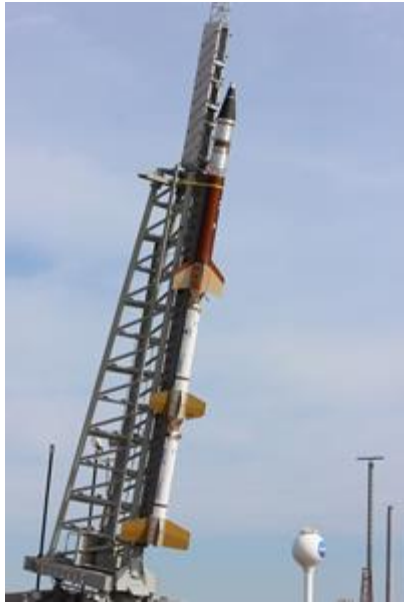
Terrier-Terrier-Oriole Sounding Rocket undergoes preparations for flight from the NASA Wallops Flight Facility, Virginia
