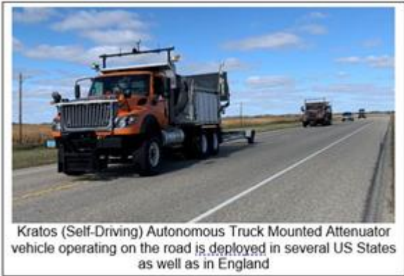
Kratos (Self-Driving) Autonomous Truck Mounted Attenuator vehicle operating on the road is deployed in several US States as well as in England
