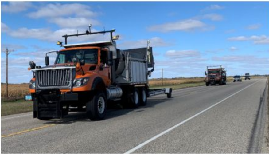
Kratos (Self-Driving) Autonomous Truck Mounted Attenuator vehicle operating on the road is deployed in several US States as well as in England
