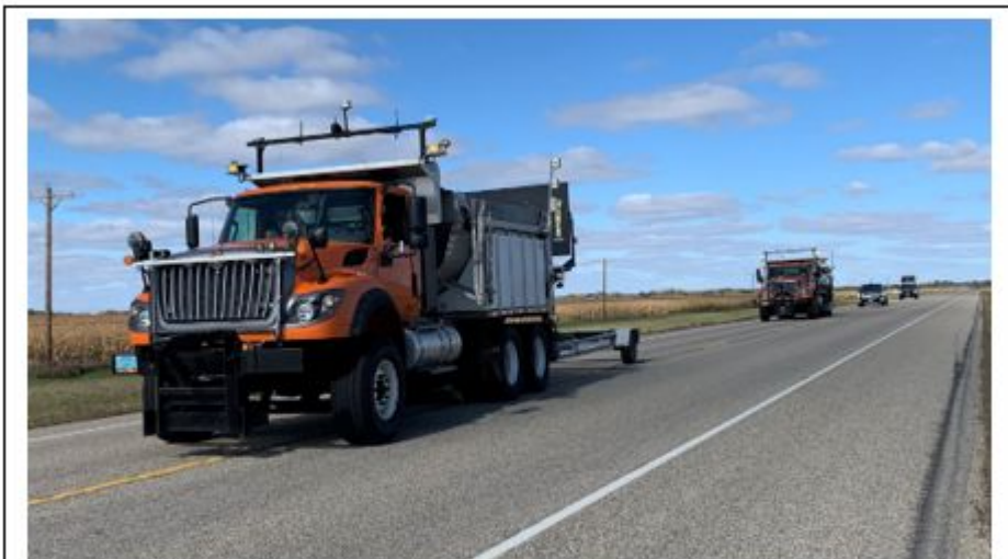
Kratos (Self-Driving) Autonomous Truck Mounted Attenuator vehicle operating on the road is deployed in several US States as well as in England
