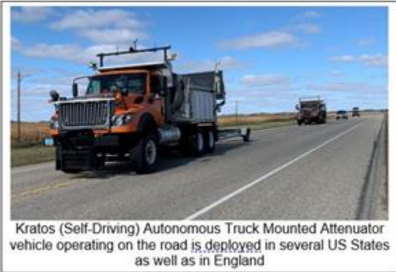
Kratos (Self-Driving) Autonomous Truck Mounted Attenuator vehicle operating on the road is deployed in several US States as well as in England
