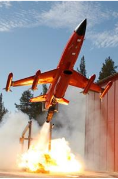
BQM-167 with full suite of external payloads - wing station and wingtip for broad range of threat replication and countermeasures
