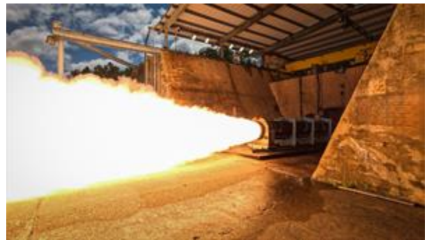
Zeus 2 Solid Rocket Motor Fires During April 10th Static Test
