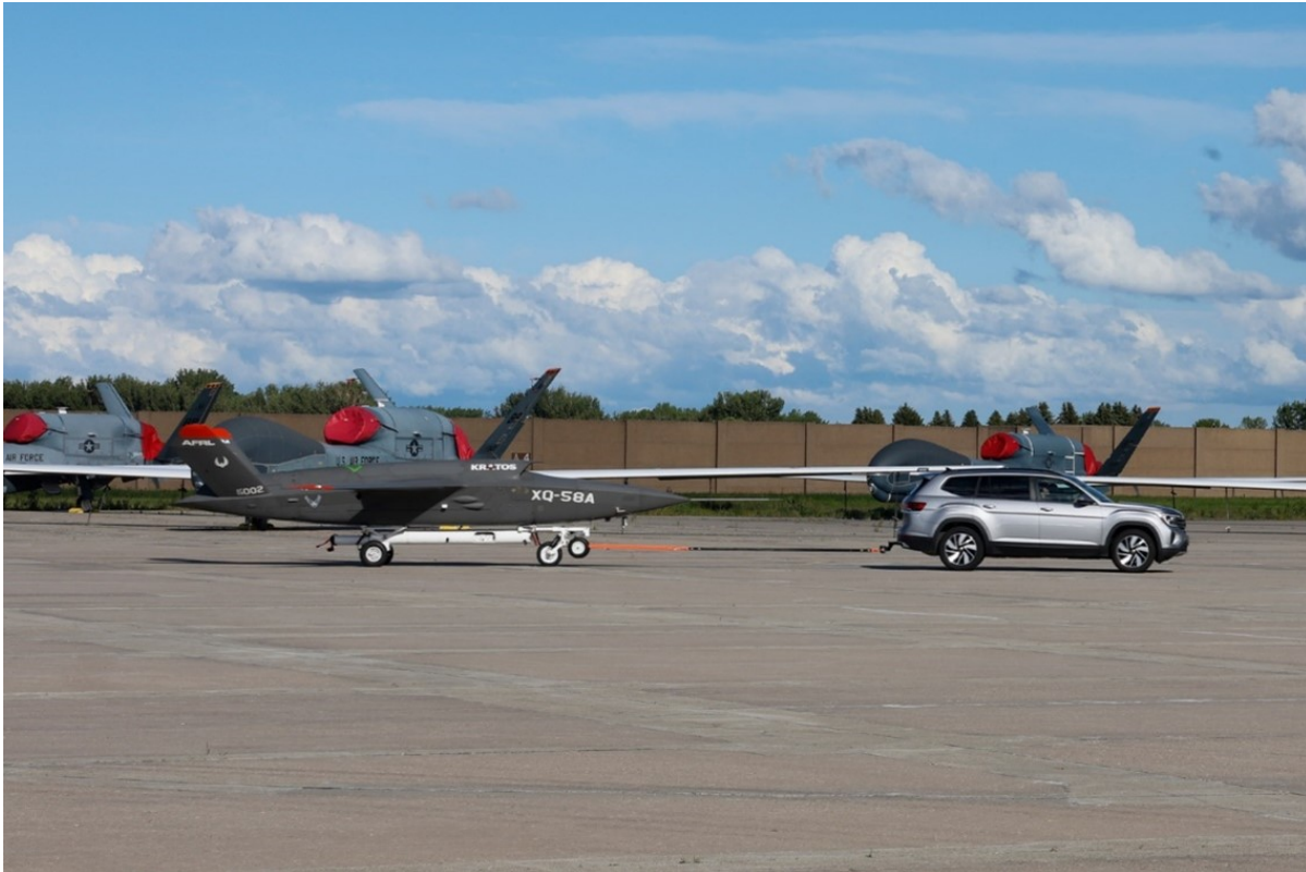
Valkyrie on KTLS Being Towed by Small Crossover Demonstrating Affordable Approach to Support Systems and Maximum Flexibility of Operations
