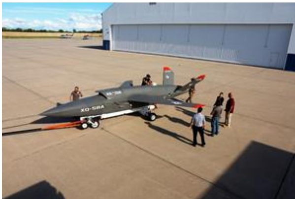
Kratos Valkyrie on KTLS Before Being Towed out to Runway for Takeoff
