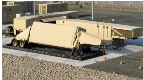
THAAD AN/TPY-2 Radar Electronic Equipment Unit (EEU)
