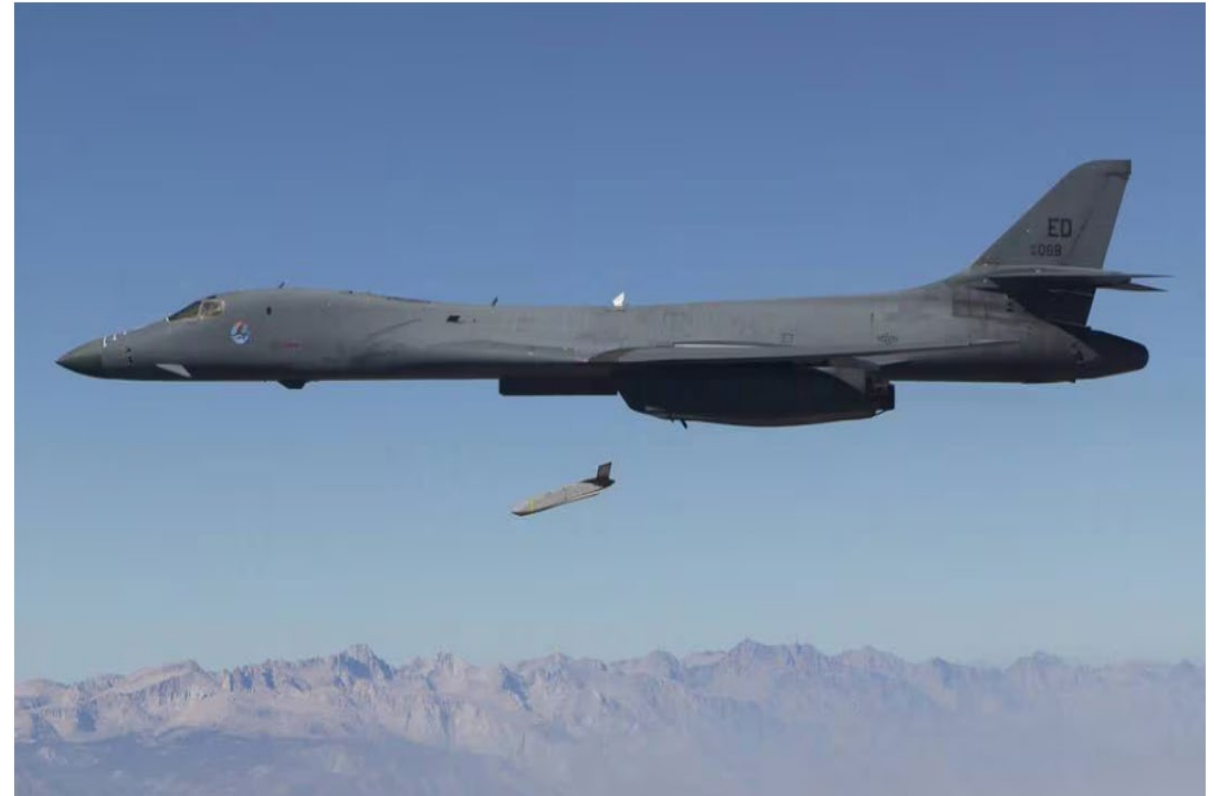
A Long Range Anti-Ship Missile (LRASM) launches from an Air Force B-1B Lancer during flight testing in August 2013. (DARPA)
